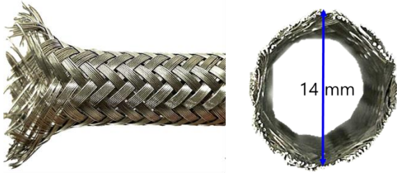
Fig. 2. Side and cross-sectional views of the braided wire wick in this study.
