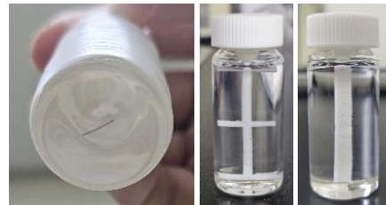
Fig. 2. ^{60}\text{Co} radioactive source in the \beta detector (left) and holders for testing position dependence (center and right).
