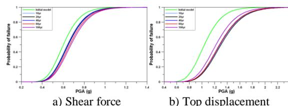
Fig. 3. Fragility curve of RC shear wall according to failure criteria
