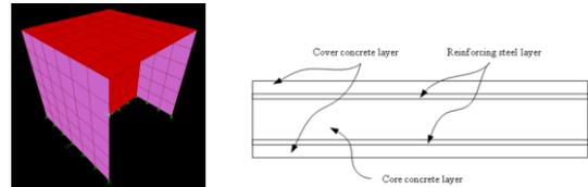
a) Finite element model b) Multi-layered shell element
