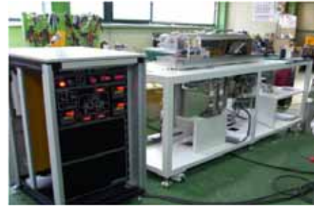
Fig.1. Apparatus for suction transport experiments.
