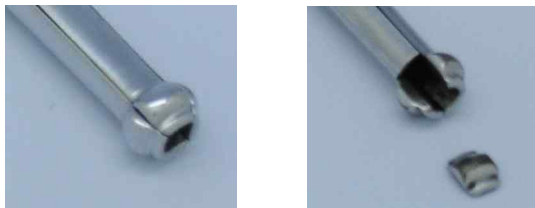
(a) standard state (b) fracture state Fig. 2. Fracture of the bulge tool
