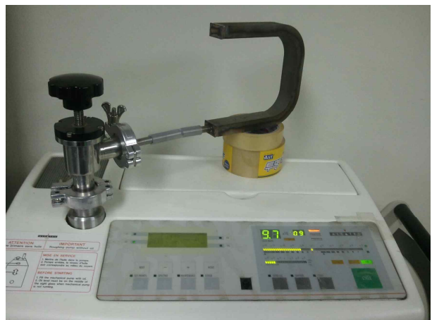
Fig. 3. Helium leak test of a welded block of a U-type small mock-up
