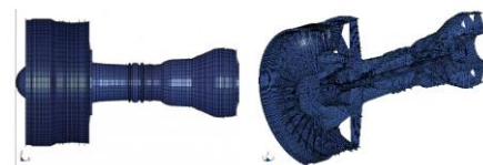
Fig 1. FE model of PW4000-96 proposed by NIST[3].
