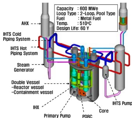
Fig. 1 Concept of Sodium-Cooled Fast Reactor
