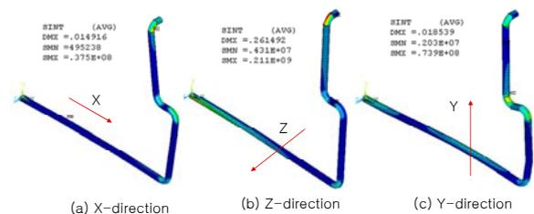
Fig. 2 Seismic Stress Responses
