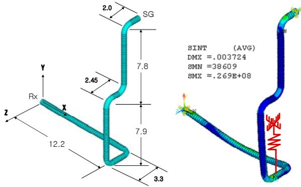
Fig. 3 IHTS Hot Pipe Layout Fig. 4 Support Location
