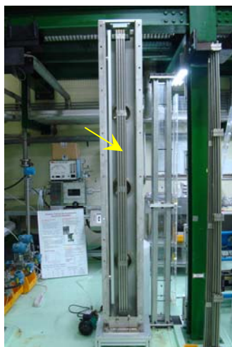
Fig. 1 4x4 dual-cooled partial fuel test assembly mounted on the UMAP.
