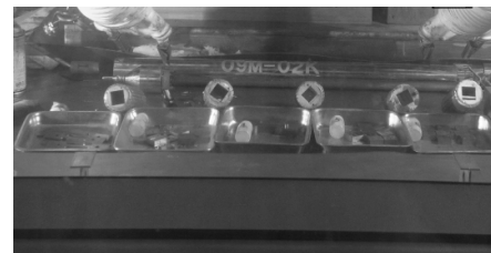
Fig. 1 The cutting machine in a hot cell
