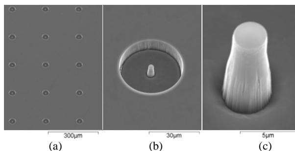
Fig. 1. SEM image of SiC micropillar array, (a) part of 20 $\times$ 20 array, (b) one crater with a pillar at the center, (c) magnified image of a pillar
