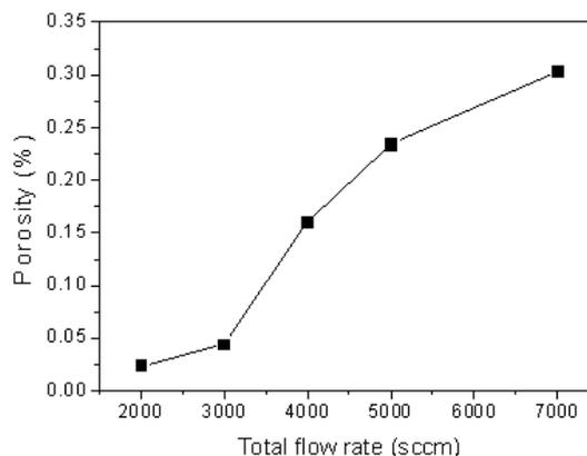
Fig. 4. Porosity of SiC layers deposited at various gas flow rates.
