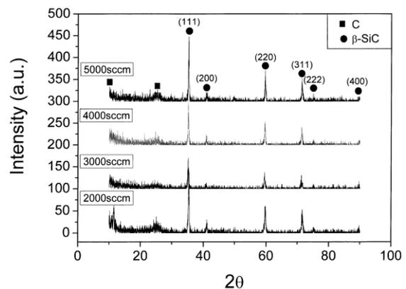
Fig. 1. XRD patterns of SiC layers deposited at various gas flow rates.
