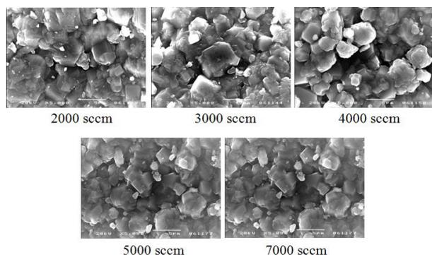
Fig. 2. SEM microstructures for the surfaces of SiC layers deposited at various gas flow rates.
