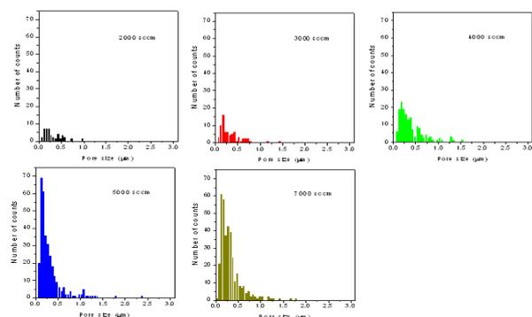
Fig. 3. Pore size distribution of SiC layers deposited at various gas flow rates.
