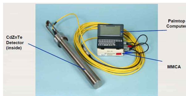
Fig. 1. IRAT : Irradiated Fuel Attribute Tester
