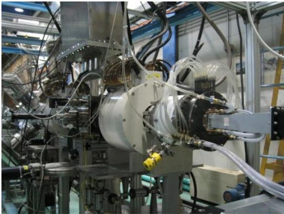
Fig. 1: Microwave ion source installed at PEFP 20-MeV proton accelerator.
