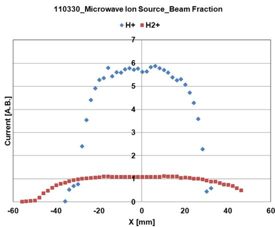
Fig. 3: Beam current signal profile of the two species ( $H^+$ ,  $H2^+$ )
