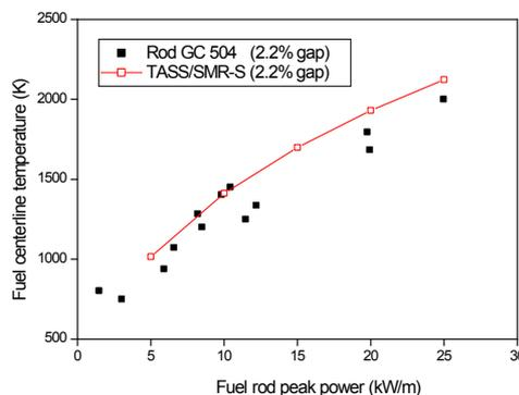
Fig. 4. Fuel center temperature (filled with argon).
