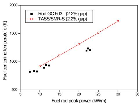
Fig. 2. Fuel center temperature (filled with Helium).
