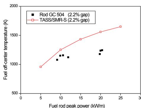
Fig. 5. Fuel off-center temperature (filled with argon).
