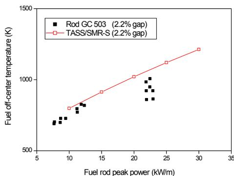
Fig. 3. Fuel off-center temperature (filled with Helium).
