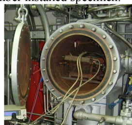
Fig. 5 DBE simulation chamber installed specimen
