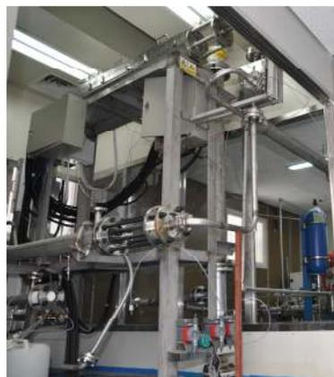
Fig. 1. Small Scale Sulfuric Acid Loop
