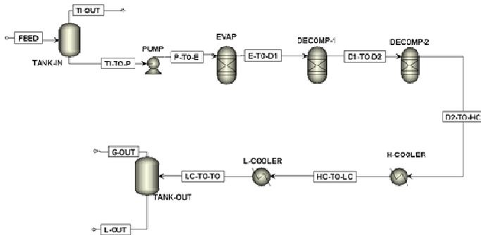
Fig. 2. Flow sheet of the sulfuric acid loop for Aspen+ modeling
