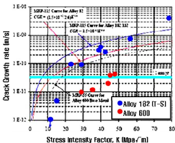
Fig. 3 The CGR values of the Alloy 600 base metal and the Alloy 182 weld metal, depending on the stress intensity factor.
