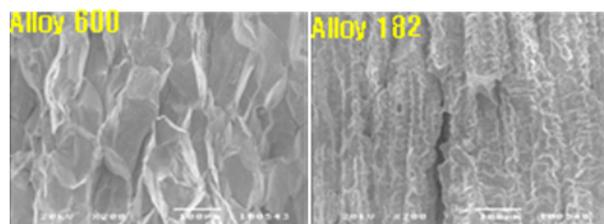
Fig. 4 Fracture surfaces of the Alloy 600 base metal and the Alloy 182 weld metal.
