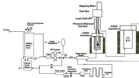
Fig. 1 Schematic diagram of the PWSCC test loop.
