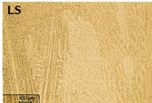
Fig. 2 Optical micrograph taken in the Alloy 182 weld metal.
