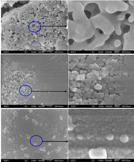
Fig. 4. FE-SEM image of virgin SAP(top), product(mid) and consolidated form(bottom) with 25wt% mixing ratio of glass.
