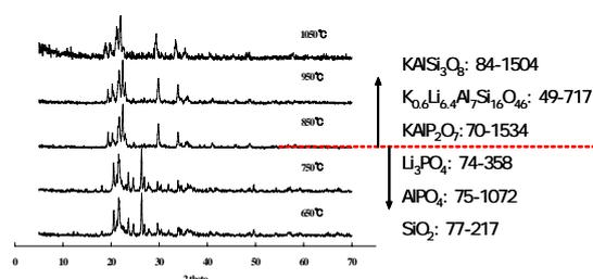
Fig. 1 XRD patterns of reaction products heat-treated at different temperature.
