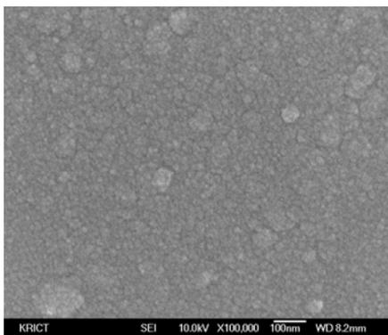
Fig. 5 FE-SEM image of consolidated form with 35wt% mixing ratio of glass
