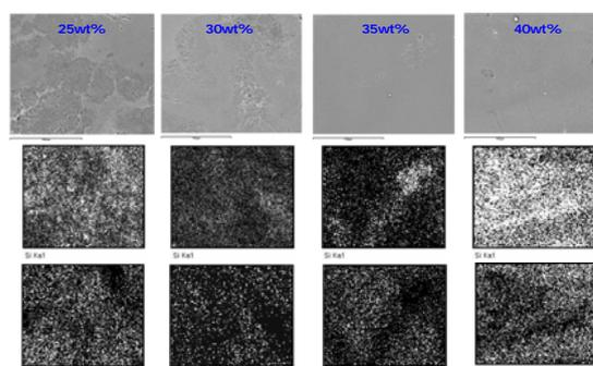
Fig. 3 SEM image and element mapping image (top: Si, bottom: P)
