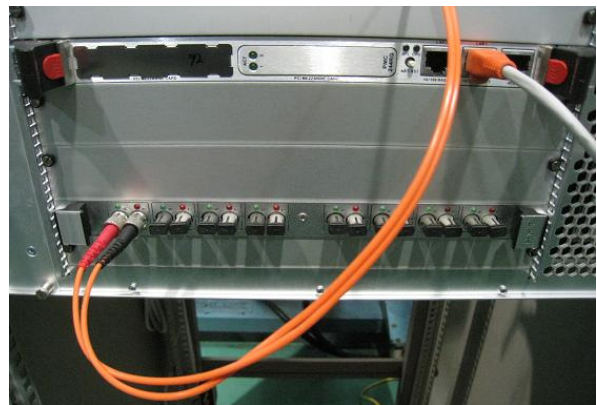
Fig. 2. Serial to optical fiber VME I/O board
