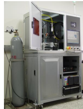
Fig 2. Photograph of the Fiber laser welder.
