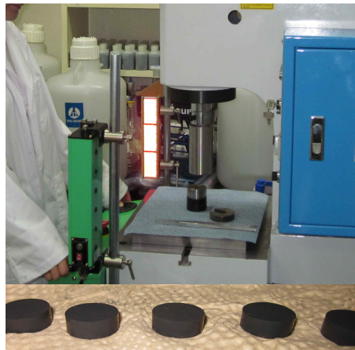
Fig. 2. A Researcher is Making Simulated Sludge Pallets by Using a Hydraulic Press and a Mold
