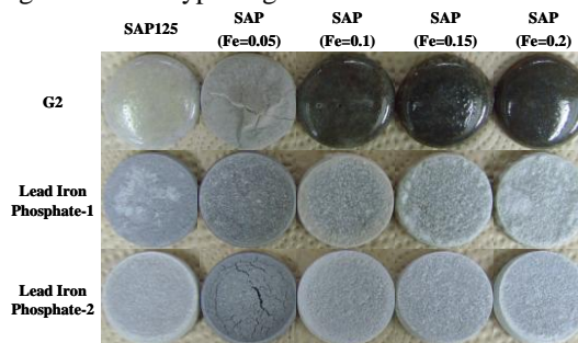
Fig. 4 Photographs of consolidated forms prepared by using different glass.
