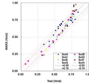
Figure 2. Comparison of MARS predicted and measured void fractions
