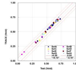
Figure 3. Comparison of TRACE predicted and measured void fractions
