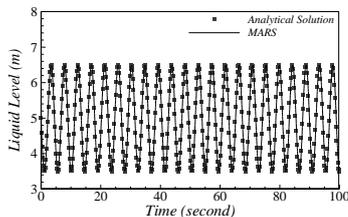
Figure 1. Variation of liquid level for the manometer problem
