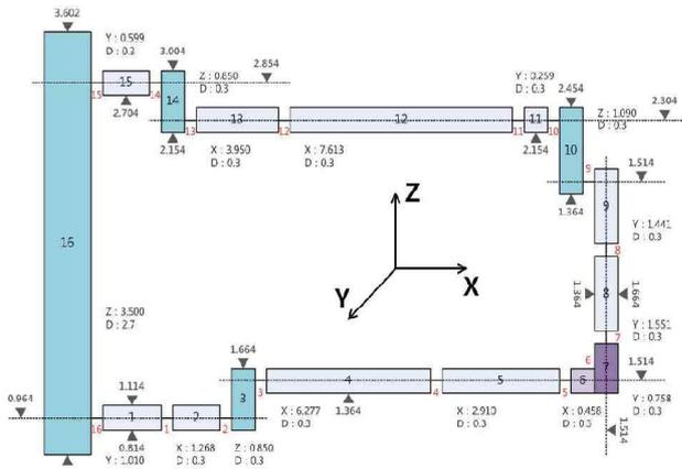
Fig. 2 Nodalization of Test Loop.
