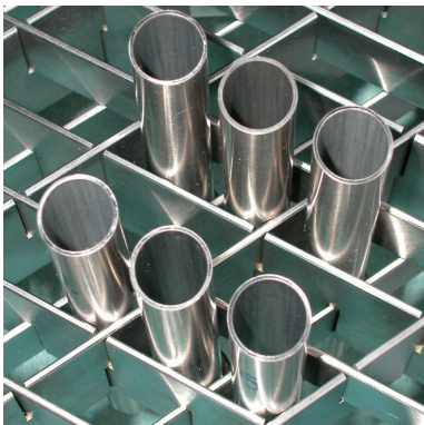
Figure 1. Mockup assembly of steam generator tubes with OD axial crack and eggcrate.
