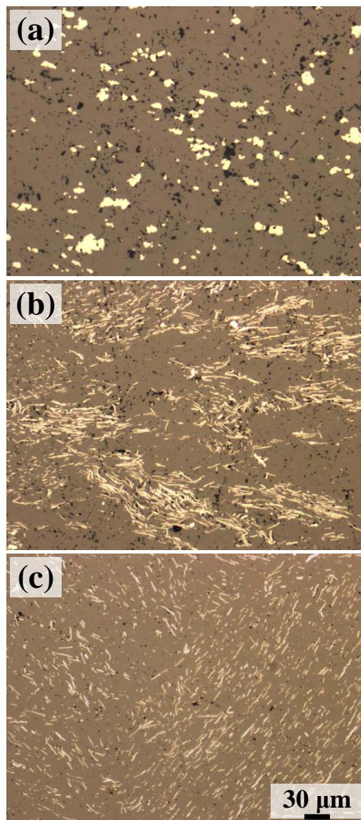
Figure 1. The optical microscopic image ( $\times 200$ ) of UO<sub>2</sub> pellets containing shape-controlled metallic phase: powder mixture milled for (a) 0 h, (b) 5 h, (c) 8 h.
