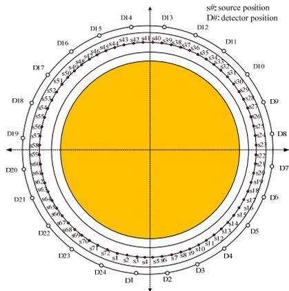
Fig. 3. Measurement geometry for riser
