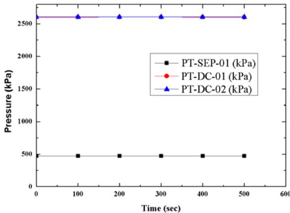
Fig. 3. The pressure changes of down-comer and separator.
