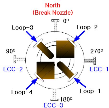
(b) Loop arrangement of main test section
