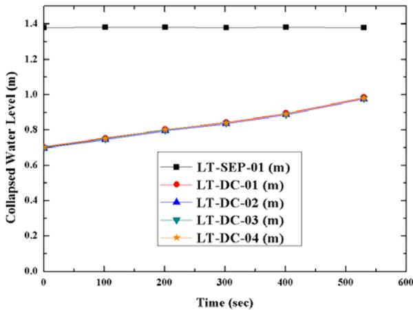
Fig. 2. The level changes of down-comer and separator.
