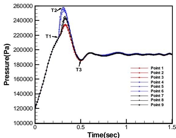
Fig. 2 Time history of pressure in end of beamtube
