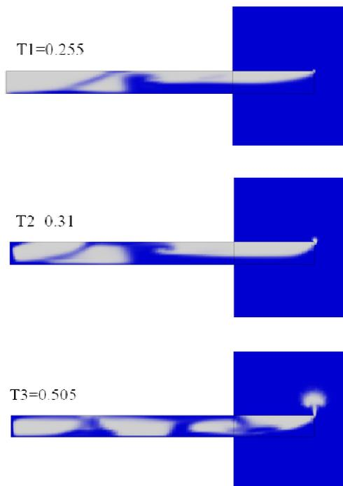
Fig. 3 Volume fraction with time variation in beamtube
