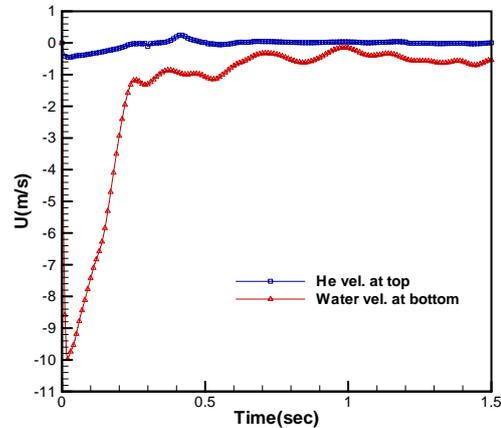
Fig. 4 Helium & water velocity with time variation in beamtube
