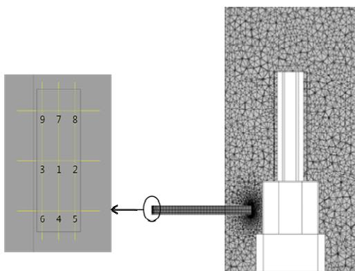
Fig. 1 Beamtube structure into pool and measurement points
