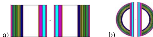
Figure 1: a) Blanket shape with cylindrical outer blanket. b) Blanket shape with spherical outer blanket.
