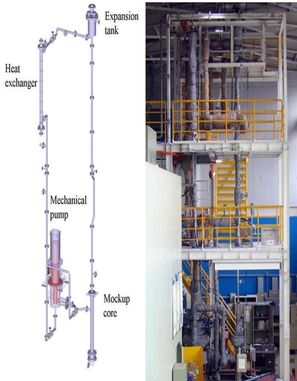
Fig. 1. 3D CAD drawing of HELIOS and picture located in the NUTRECK, Seoul National University
