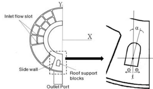
Fig. 1. Geometrical parameters in Outlet Plenum of PBMR; displacement on the horizontal line ( $l$ ) and angle of rotation ( $\alpha$ ) about the center of gravity of the roof support block.
