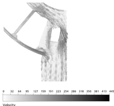
Fig. 2. Velocity vectors around the roof support block for the reference case
