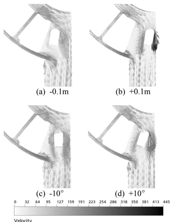
Fig. 3. Velocity vectors around the roof support block for different values of  $l$  and  $\alpha$
