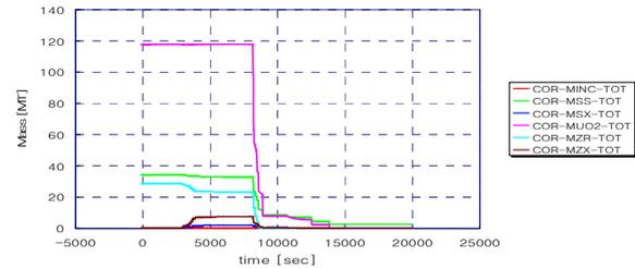
Figure 2. Total Mass of Core Materials melted and ejected to cavity in LBLOCA with MELCOR Version 1.8.5
