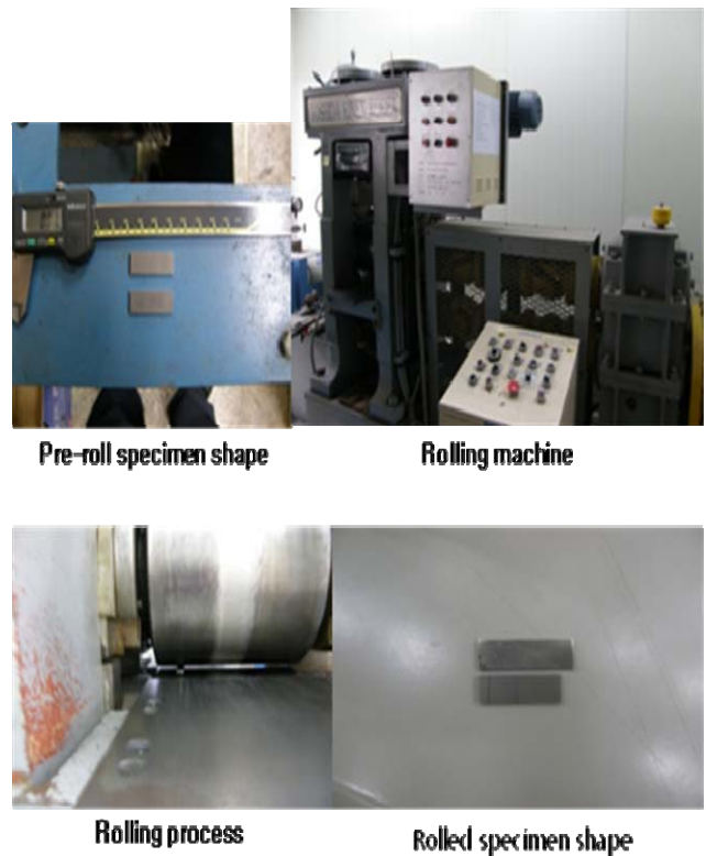
Fig 1. Rolling specimen preparation process
