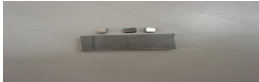
Fig 2. Machined specimen for DSC
