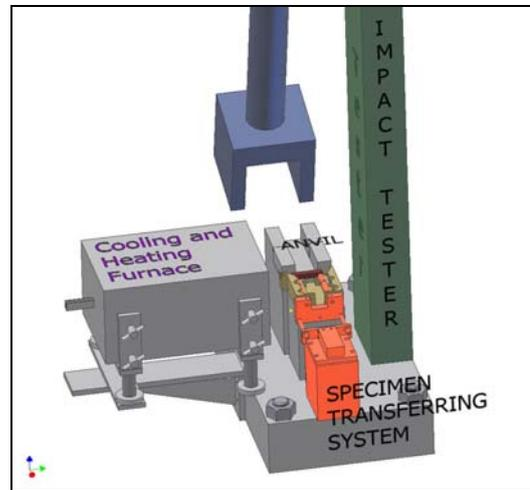
Fig. 1. 3-D view of a remote-controlled impact test system in IMEF.
