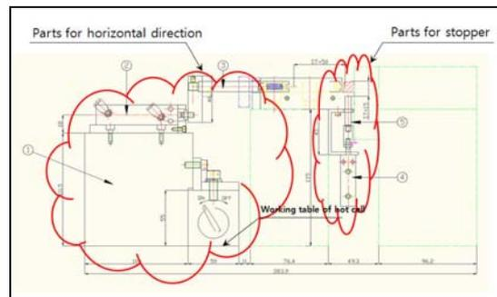
Fig. 2. Elevation View of an Advanced specimen transferring device with both parts for horizontal direction and for stopper.
