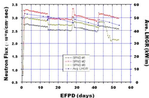
Fig. 5. Neutron flux during the irradiation test in the OR5 hole of HANARO.
