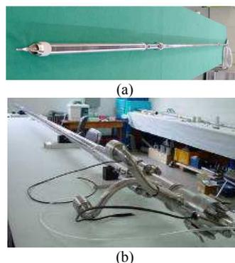
Fig. 2. (a) Instrumented capsule for nuclear fuel irradiation testing and (b) In-pile section of fuel test loop.
