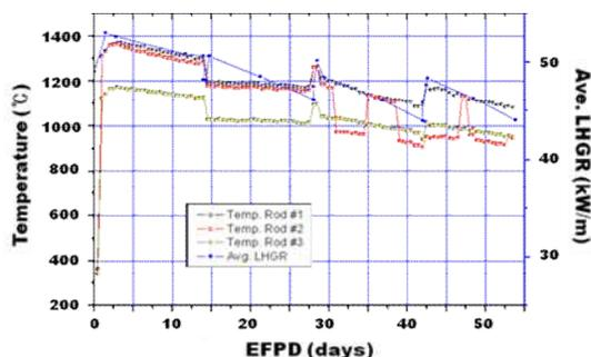
Fig. 3. Central temperature of nuclear fuels during the irradiation tests.
