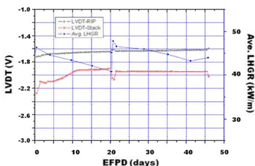
Fig. 4. Variation of data from LVDTs during the irradiation test in the OR5 hole of HANARO.
