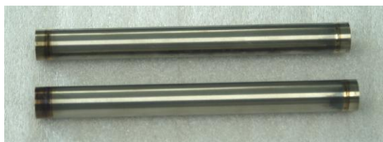
Fig. 3. Fabricated creep specimens for the simulated dual-cooled cladding tube.
