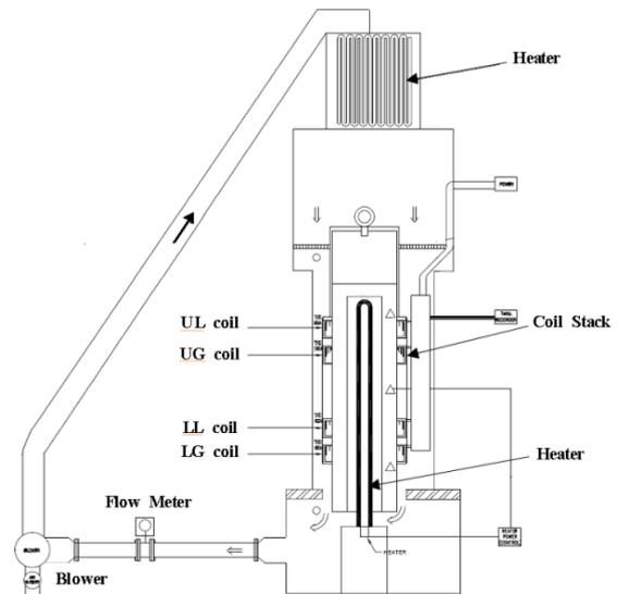
Fig. 1. Cooling performance test facility
