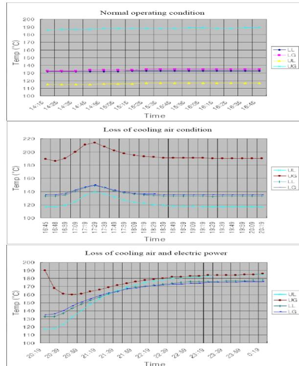
Fig. 3. Temperature traces of 4 CEDM coils
