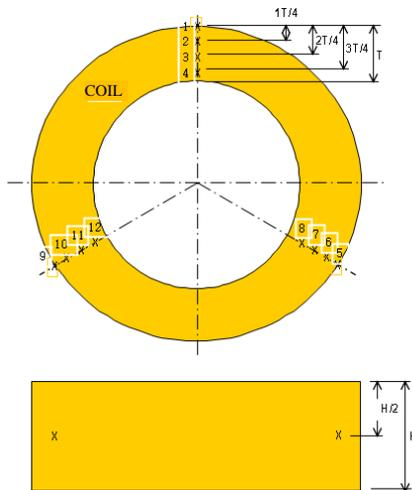
Fig. 2. Thermocouples (marked "x") in the UG coil as an example. Other coils each have 6 thermocouples (at the position numbers 1, 4, 5, 8, 9, and 12).
