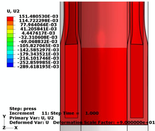
Fig. 2 Multiple plot of the un-deformed and deformed shape after the 1<sup>st</sup> step analysis.
