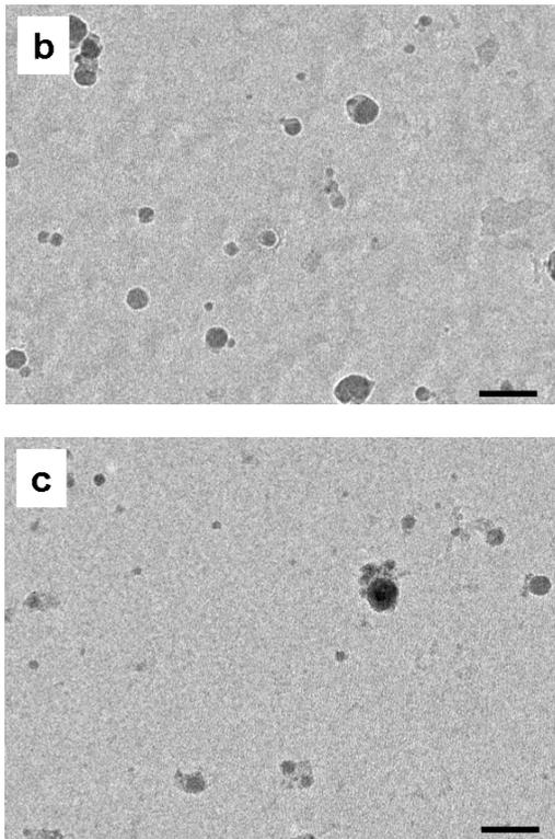
Fig. 1. Precipitates in (a) H0, (b) H1 and (c) H2 ODS steels. (Carbon extraction replica samples)
