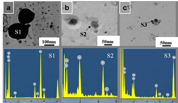
Fig. 2. EDS analysis of the precipitates in (a) H0; (b) H1 and (c) H2
