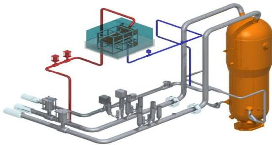
Fig. 1 Major equipment and piping of the PAFS in the APR+
