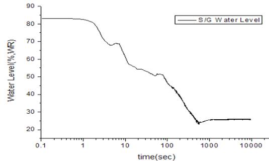
Fig3. Steam generator Water level (LOCV)
