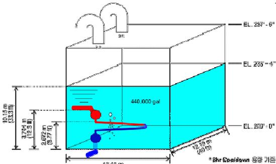
Fig. 2. Schematic diagram of PCCT in PAFS
