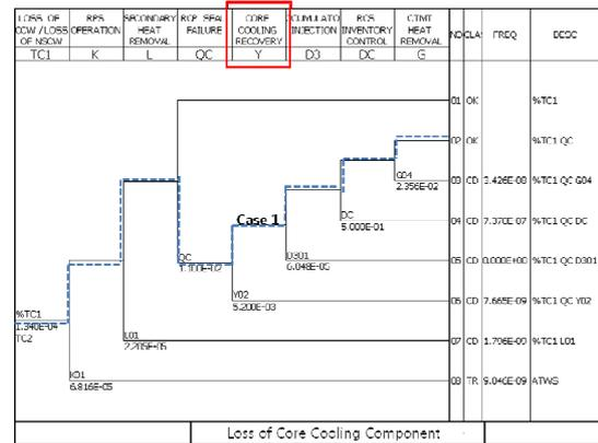
Fig. 1. Case 1 (Sequence no. 2) contains the core cooling recovery operation in the loss of CCW event tree.
