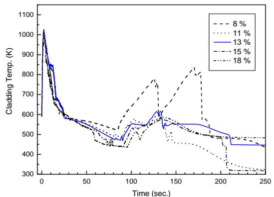
Fig.3. Cladding temperatures of the outside cladding.
