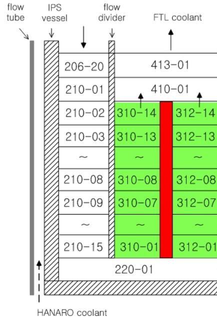
Fig.1. Modeling of the annular fuel rod within the IPS.
