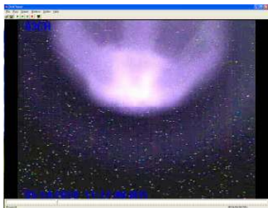
FIGURE 2. Camera image of the ECR plasma that are seen through the beam extraction hole, when trim coil current is 200 A ( B_{z\min} = 0.31 T).
