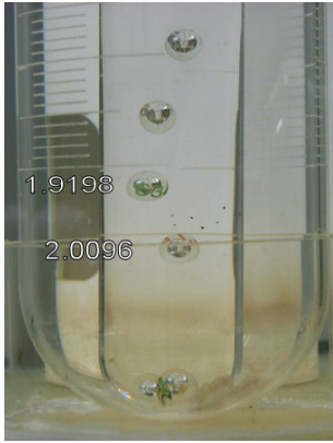
Fig.2. Standard float and O-PyC fragments floated in a density gradient column for TR225 sample batch.
