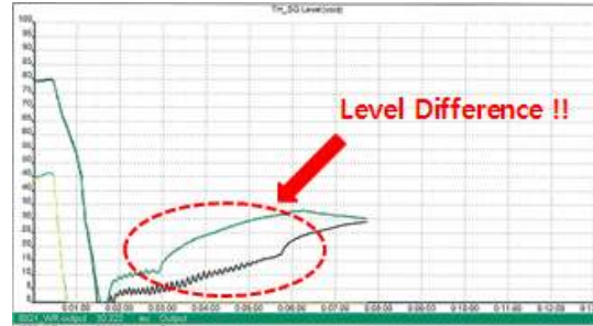
Fig. 2. SG level at feedwater head rupture(before)
