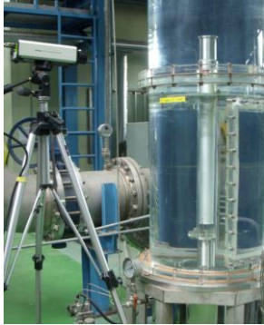
Fig. 4. Vibration Measurement using a Laser Vibrometer
