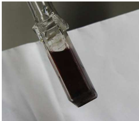
Fig. 2. Photo of uranium(III) chloride in LiCl-KCl eutectic melt
