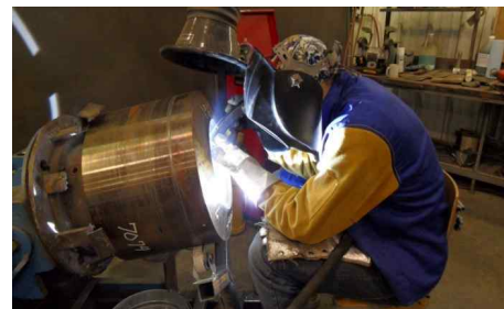
Fig. 2. Manufacturing of dissimilar metal weld test specimen
